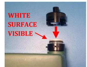
Step 3.5 Place impactor plate back in the holder ensuring white surface is oiled and aligned away from the DustCount.
