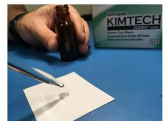
Step 3.3 Use the Impactor Oil Applicator to apply one drop of oil to a fiber-free paper pad.
