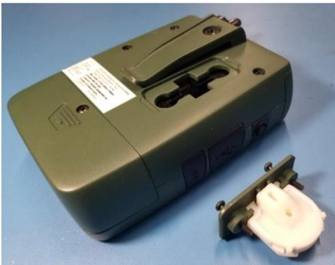
**Step 4.4** Filter cassette and filter cassette cover fully extracted from the DustCount.
