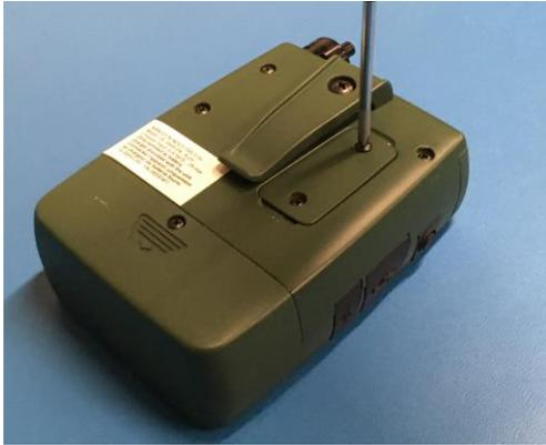
**Step 4.1** Loosen filter cassette cover screws with a small Philips screwdriver.
