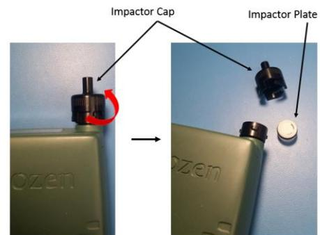
Step 3.1 Twist off Impactor cap and remove impactor plate assembly from the holder.
