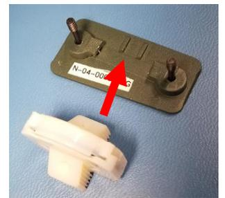
**Step 4.11** Slide filter cassette onto filter cassette cover, insert back into DustCount and tighten filter cassette screws.
