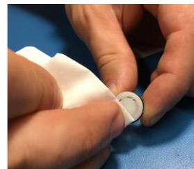
Step 3.2 Use a fiber-free cloth (Kimwipes) soaked in alcohol to remove any visible dust on the white porous surface.
